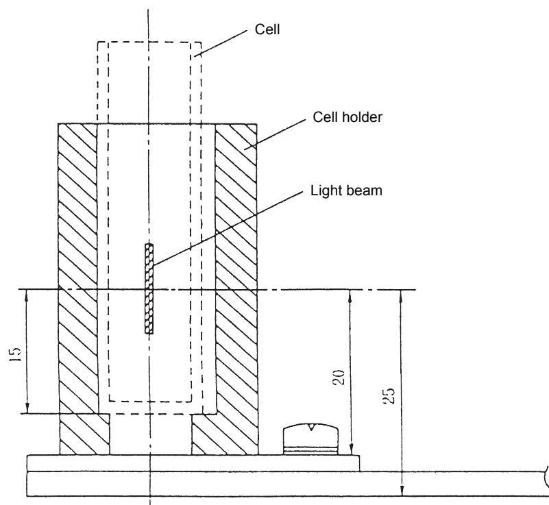
[Fig.7-17 Positional Relationship of Cell Holder \(Cell\) and Light Beam "UV-2600i/2700i"](#)
