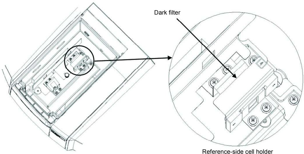
Fig.3-6 Mounting a Dark Filter onto the Film Holder
