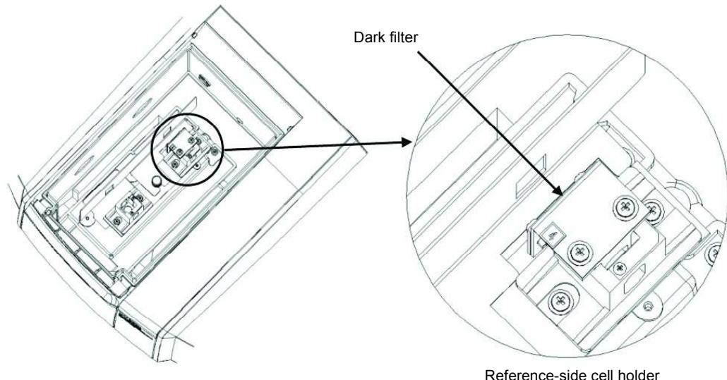
Fig.3-3 Mounting a Dark Filter
