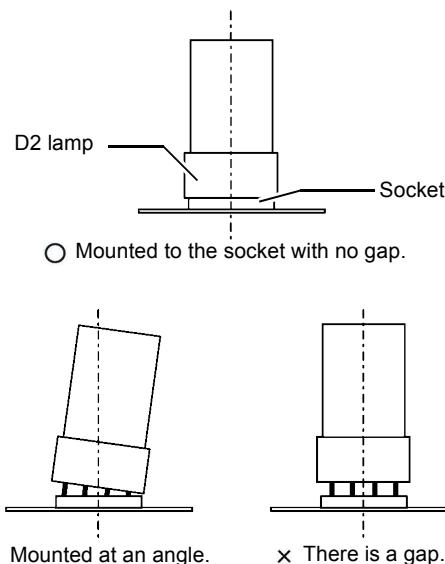
Fig.2-5 Checking D2 Lamp Installation
