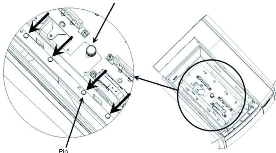
Fig.3-4 Mounting the Partition Plate onto the Rotary Film Holder
