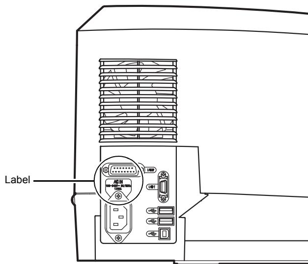
Fig.2-2 Location of the Power Supply Voltage Indication
