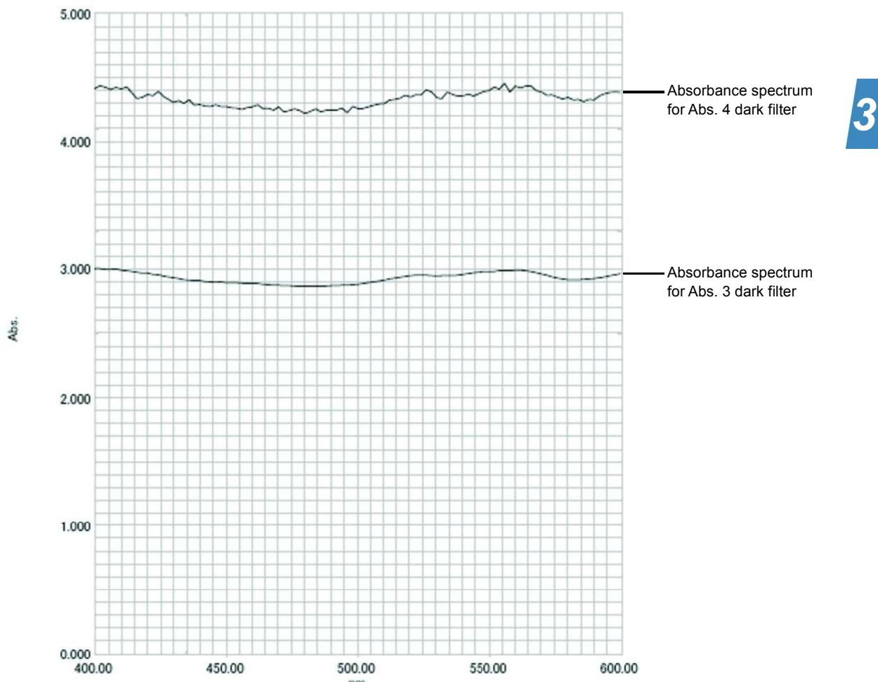
Fig.3-9 Absorbance Spectrum for Dark Filters
