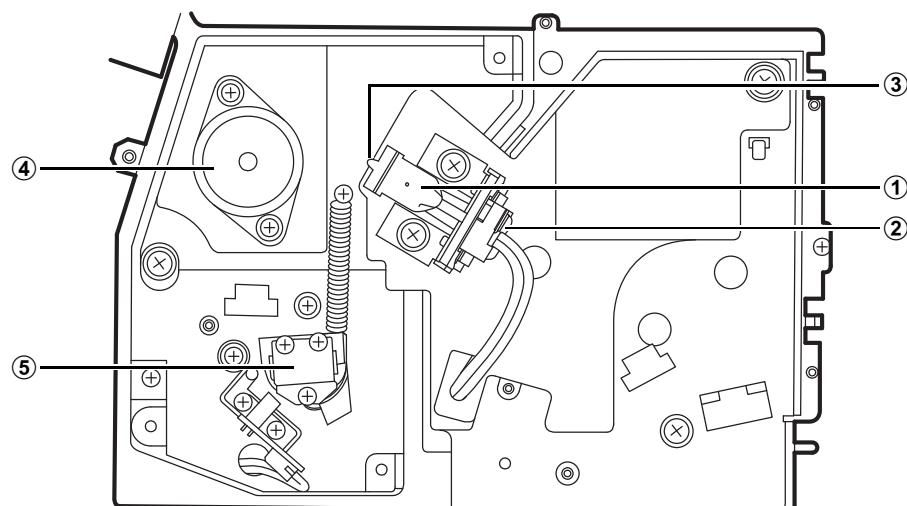
Fig.4-5 Light Source Compartment (UV-2600i)
