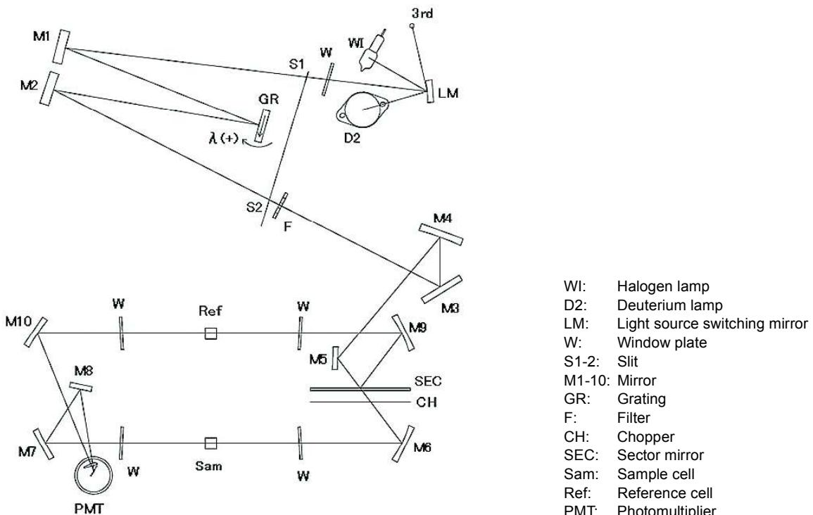
Fig. 7-16 Schematic Optical System (UV-2600i)
