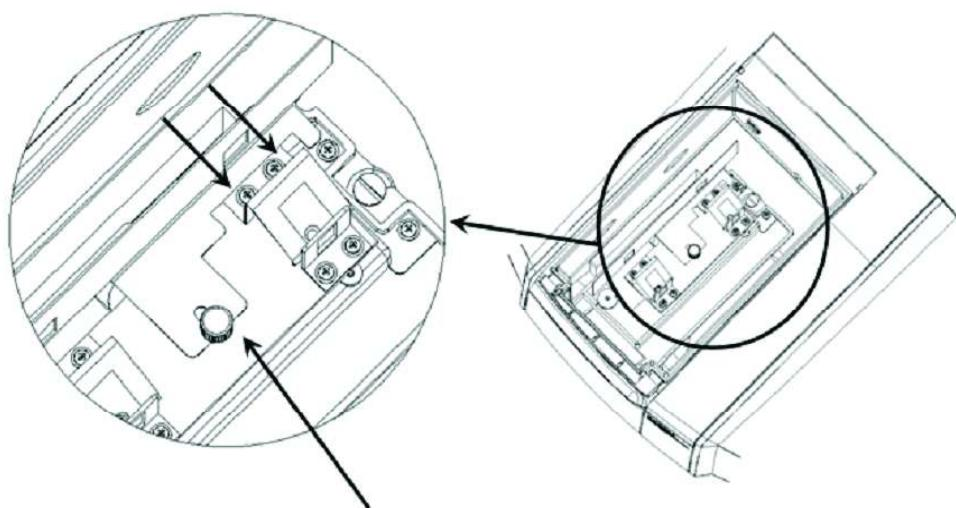
Press the partition plate against the side of the film holder on the reference side for positioning and then secure it in place with the knurled screw.
