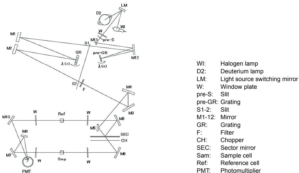
Fig.7-15 Double Monochromator Configuration (UV-2700i Series)
