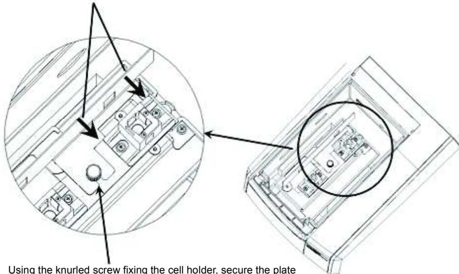
Fig.3-2 Mounting the Partition Plate
