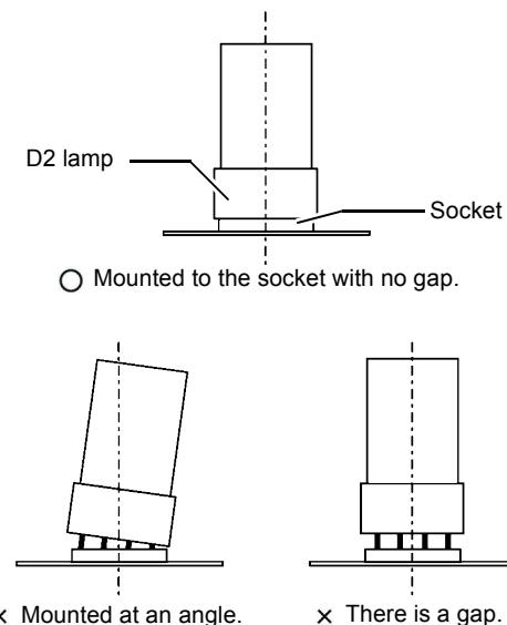
Fig.4-14 Checking D2 Lamp Installation
