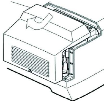
Fig.4-4 Removing the Light Source Compartment Cover
