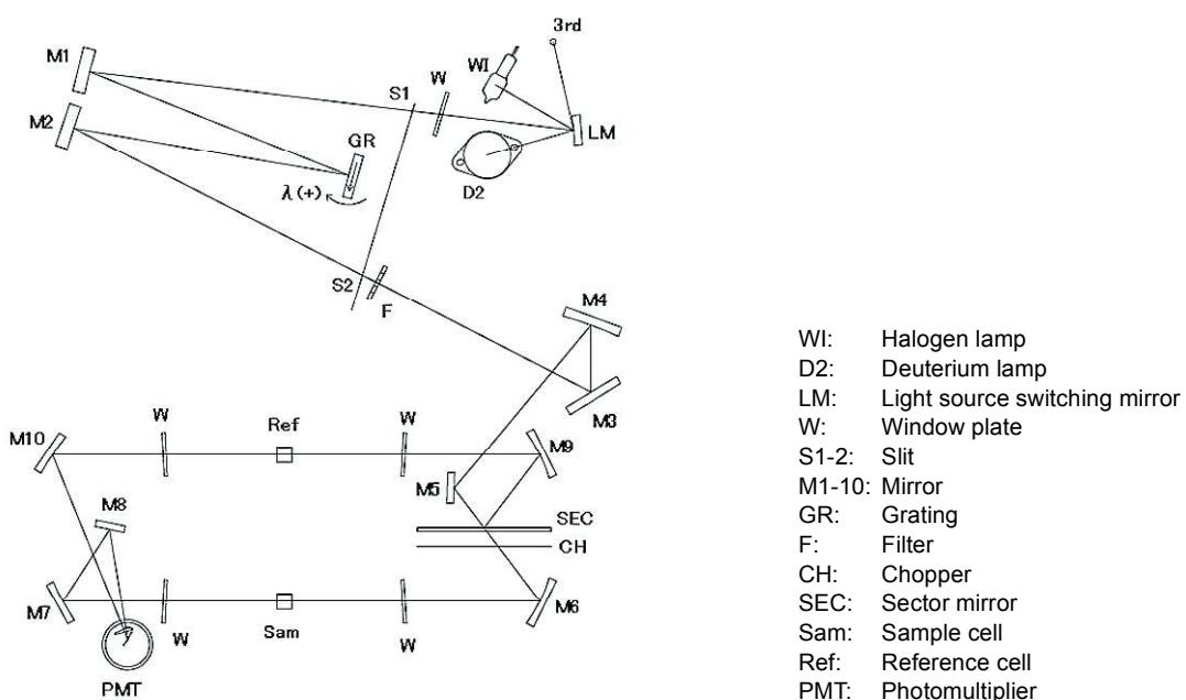
Fig.7-14 Single Monochromator Configuration (UV-2600i Series)
