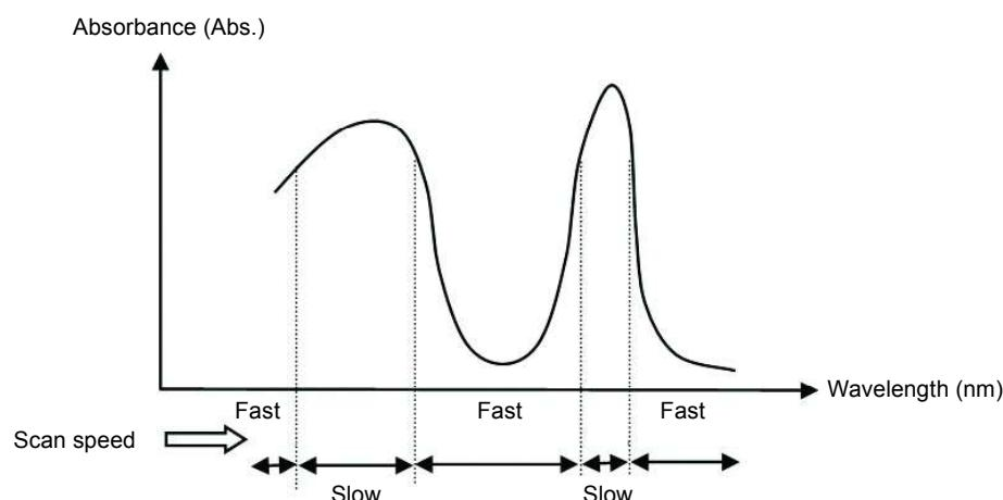
Fig.3-1 Relationship Between Absorbance Spectrum and Scan Speed in High-Absorbance Measurement Mode (Schematic)
