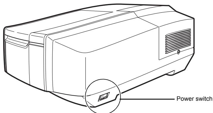
Fig.2-7 Power Switch for UV-2600i/2700i
