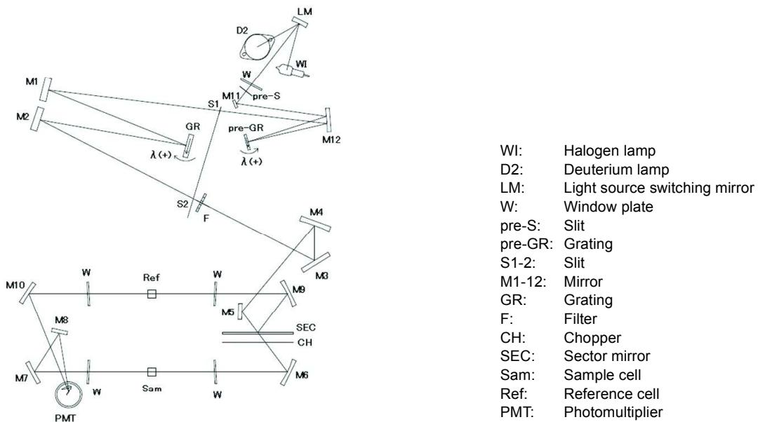
Fig.7-18 Schematic Optical System (UV-2700i)
