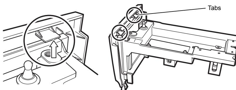
Fig.5-12 Tabs on the Sample Compartment Front Cover
