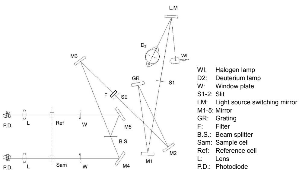
Fig.7-13 Double Beam - Double Detector Configuration
