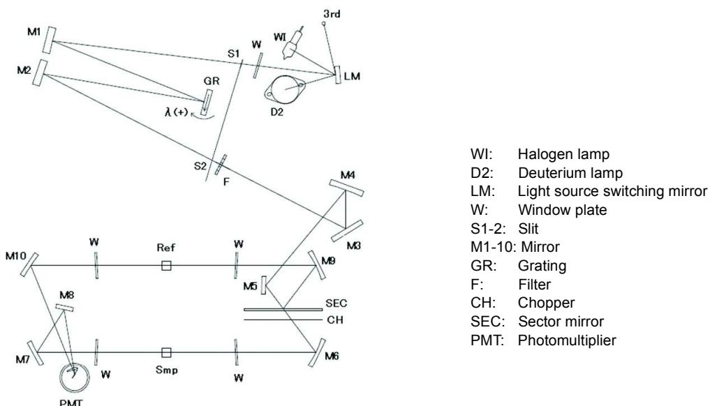
Fig.7-12 Double Beam - Single Detector Configuration (UV-2600i Series)
