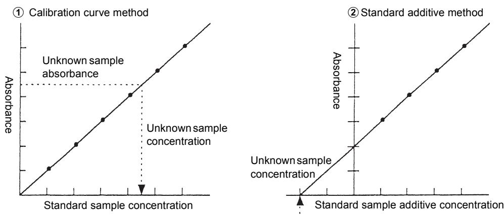
Fig.7-6 Calibration Curve
