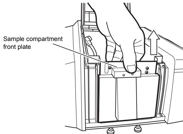
Fig.5-15 Front Plate of the Sample Compartment
