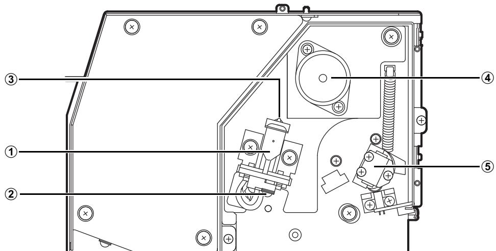
Fig.4-6 Light Source Compartment (UV-2700i)
