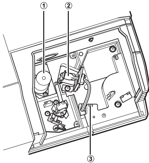
Fig.1-6 Light Source Compartment (UV-2600i)
