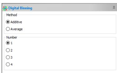
1. **Additive:** Additive Digital Binning refers to the method of combining (Adding the specified Number  $\times$  Number of pixels) pixels of blocks of neighboring same color pixels to resize the video to the lower resolution, but the higher brightness. The new resolution will be ( $Width/n$ ,  $Height/n$ , n is the Number);
