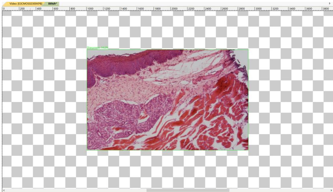
5. Move the slides with the microscope **X-Y translational control knobs** and user will see the stitching results simultaneously. Move the slide to acquire horizontal or vertical stripes. If your camera has a very wide aspect ratio (e.g. 16:10) it is recommended to scan vertical stripes. For standard aspect ratios (5:4 or 4:3) vertical and horizontal stripes are equally efficient. Make sure that adjacent stripes are overlapping by at least two rows (or columns) of grids.
