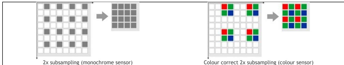
Color subsampling as performed by most color sensors, skips pixels while maintaining color. For some monochrome sensors, the camera also performs color subsampling, resulting in slight artifacts.
