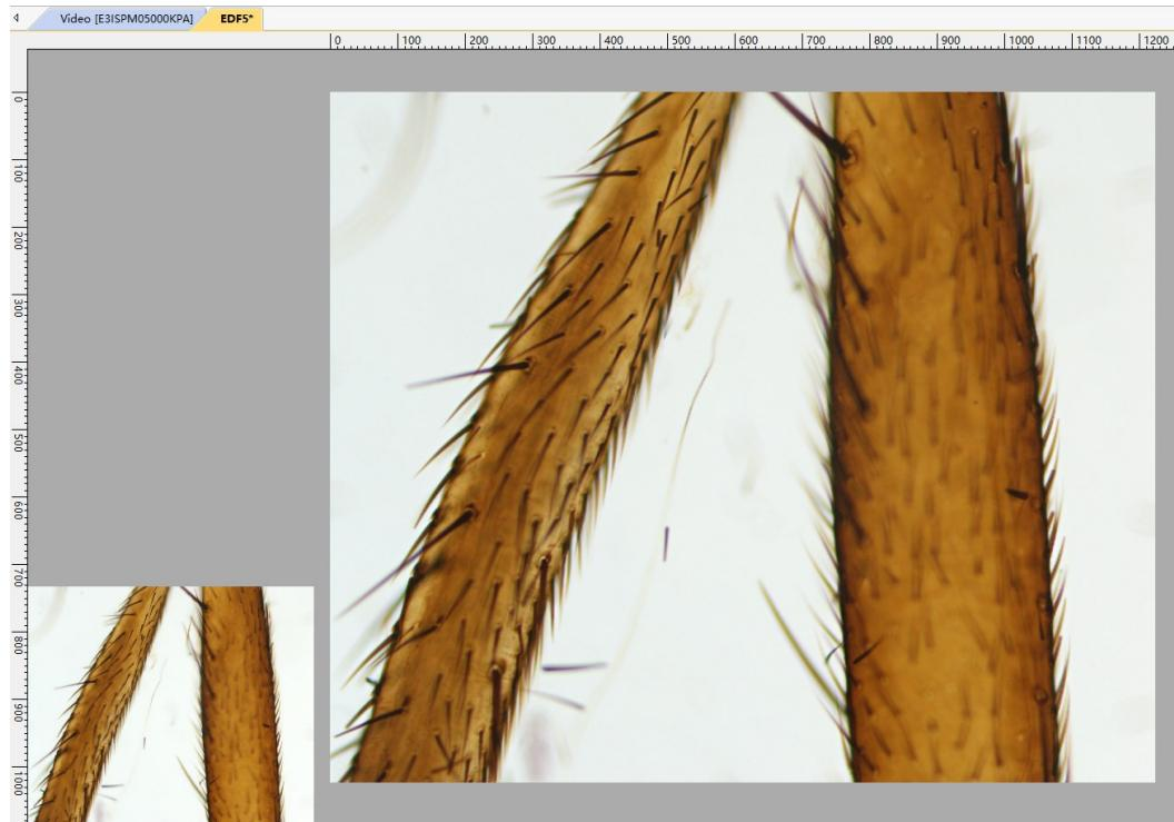
3. Rotate the microscope fine adjustment knob. The live preview of the specimen will be shown in the left bottom small video window. The **EDF** results will be updated in the right large window in real time;
