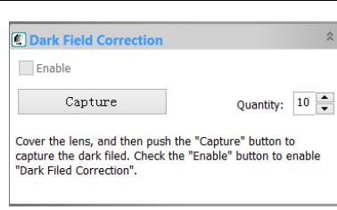
[Dark Field Correction](#) is normally used to remove the background noise or fixed pattern noise. [Dark frames](#) must be taken with no illumination.
