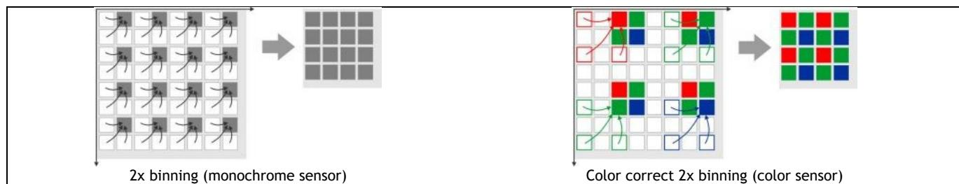
Color binning as performed by most color sensors, combines only pixels of the same color. For some monochrome sensors, the camera also performs color binning, resulting in slight artifacts.
