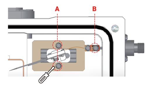
2. Disassemble the bolt A(M2x5mm) and B (M2x3mm).
