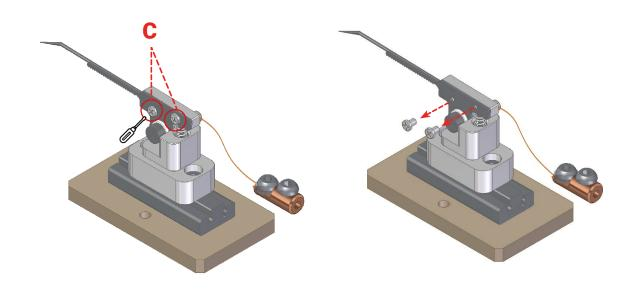
**6.** Replace a new probe tip into the groove of part D. Reassemble bolt C(M1x1.5mm).
