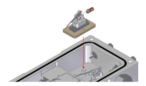
10. Tighten the bolt A (M2x5mm)Reassemble the BeCu connector to the SMA feedthrough and tighten the bolt B (M2x3mm)again
