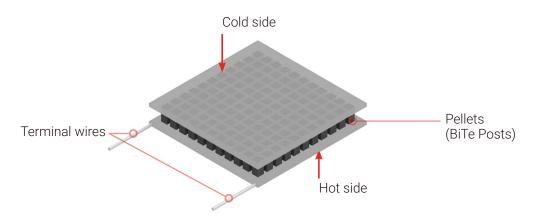
To lower the temperature of the Peltier sample stage to -40 °C, must maintain the hot side of the Peltier sample stage at  $^{1)}$  approximately under 5 °C (the required temperature is depending on a sample and measurement environment).
